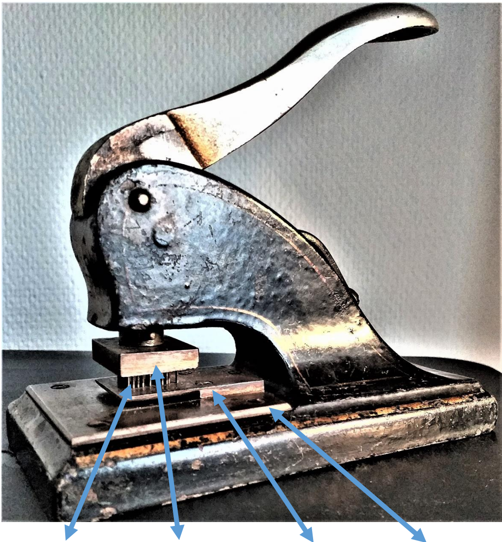
Perforeringsnåle, De to øvre matricer, Matricestyrelade, Bundmatriceplade
